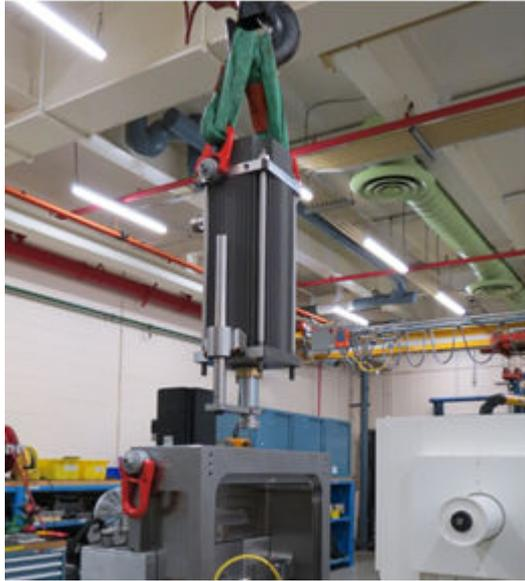
**Figure 5-13: Installing the Servo Linear Actuator**
