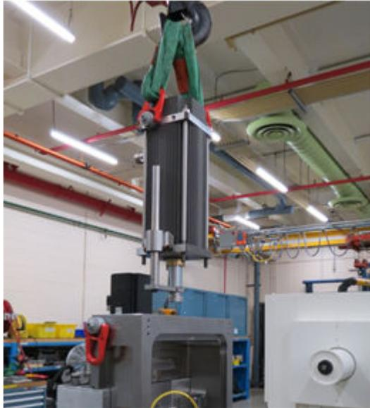
**Figure 5-11: Removing the Servo Linear Actuator**
