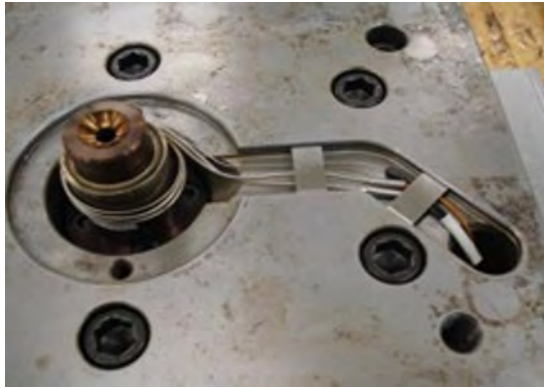
Figure 5-23: Wire Wrapped Around Sprue Heater (Example)
