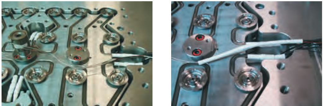
Figure 5-24: Fiberglass Sleeving (Example)
