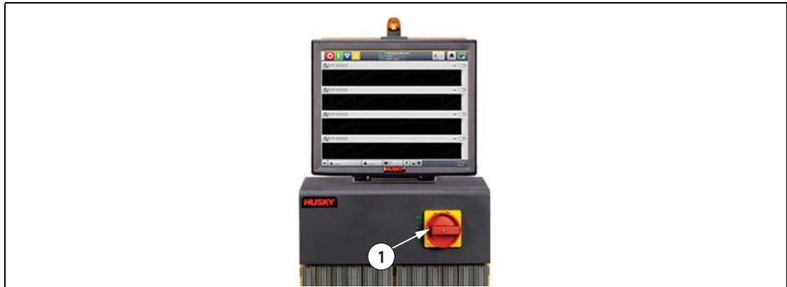
Figure 15-7 Altanium Main Power Switch
