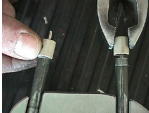
Figure 6-43: PEEK Bushing Removal and Installation
