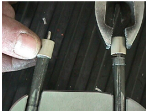
Figure 6-97: PEEK Bushing Removal and Installation
