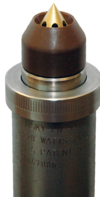
Figure 6-61: Seating the Nozzle Tip Insulator (Example)
