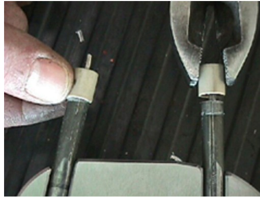
Figure 6-73: PEEK Bushing Removal and Installation
