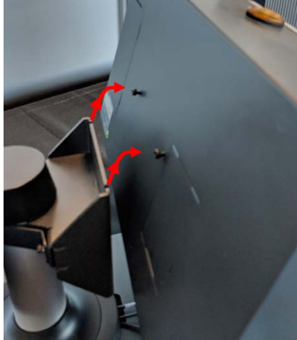
Figure 15-20 Remove the MCU from the Bracket
