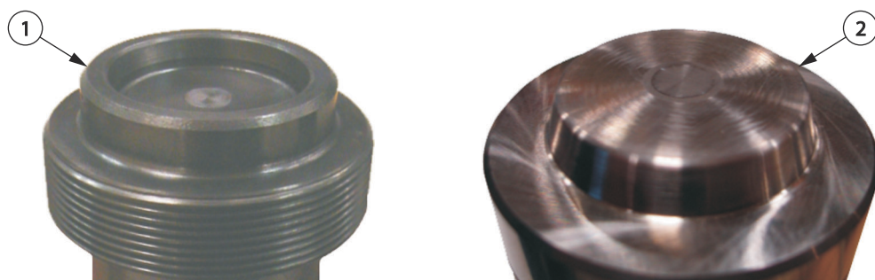
Figure 7-53: Valve Stem Protrusion
