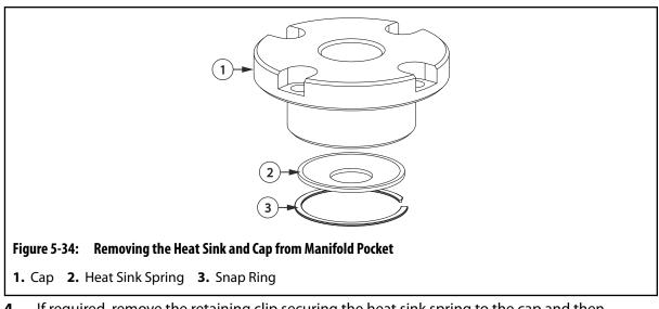
**4.** If required, remove the retaining clip securing the heat sink spring to the cap and then remove the heat sink spring.
