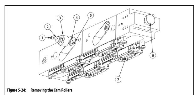
1. Screw 2. Outer Washer 3. Cam Roller 4. Inner Washer 5. Cam Shaft 6. Load Cell Adapter 7. Linear Bearing
