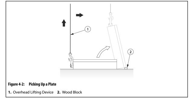
3. Lift the plate until it touches the secured wood block.
