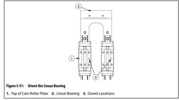
**2.** Install one linear bearing onto each of the linear rails. The plastic guard will be pushed out as the bearing moves onto the rail. This should prevent any bearings escaping the race.
