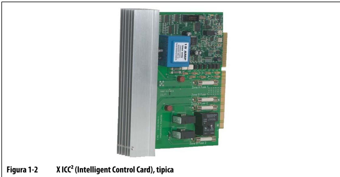
Figura 1-2 X ICC<sup>2</sup> (Intelligent Control Card), tipica
