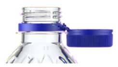
This closure was produced for a standard PCO 1881 neck finish that features a large diameter support ledge. An integrated groove within the closure shell allows it to be locked in place without interference from the support ledge.
