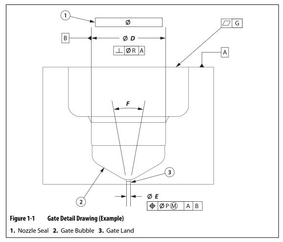
**NOTE:** The job specific gate detail drawing provides the required tolerances.
