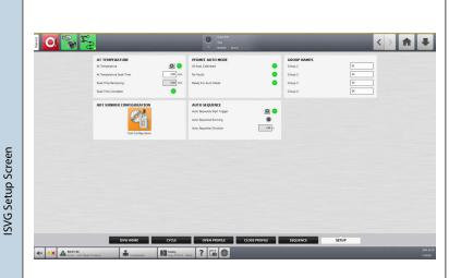
The ISVG Setup screen is used to configure the servo axes, which includes the following:
