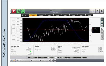
The ISVG Open Profile screen is for configuring the open profile for all or selected valve gates, which includes the following:
