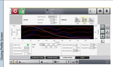
Used for configuring and plotting the speed and force profiles for the stem closing motion
