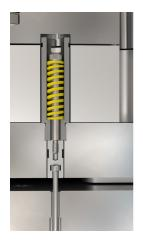
Valve-Stem open Engaged in system
