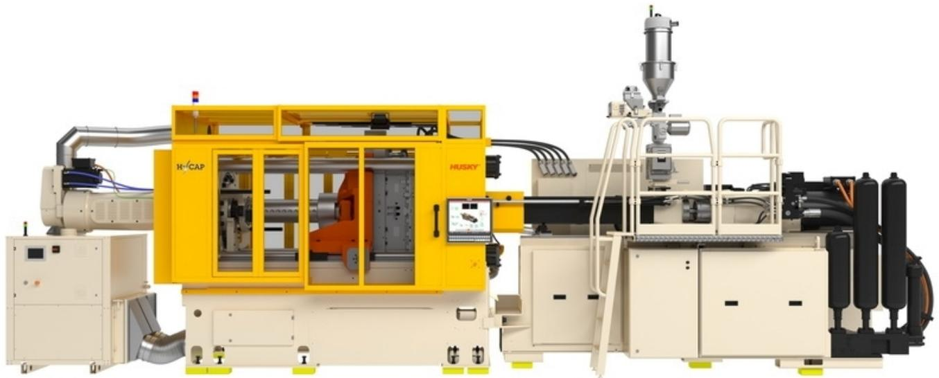
HyCAP™4 is the industry's only fully integrated beverage closure system designed and built to work together for increased productivity, energy efficiency and ease of use.
