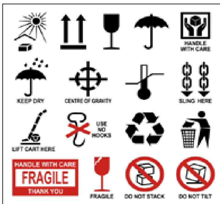
Figure 7: Package Handling Markings (DIN 55402 and ISO R780 standards)
