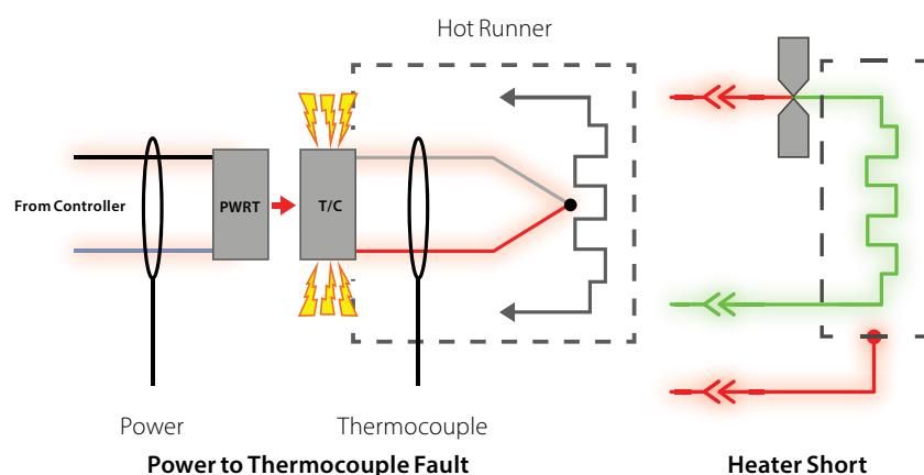
Power to Thermocouple Fault
