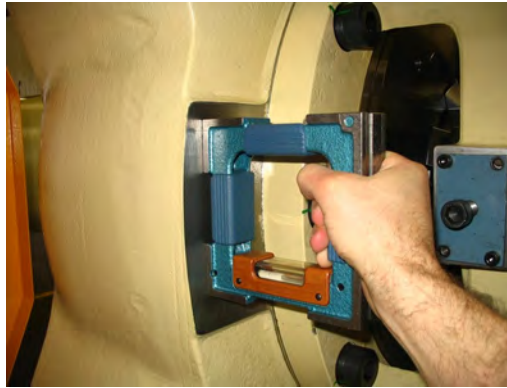
Figure 5-37: Box Level Measurement on Clamp Casting (L7)
