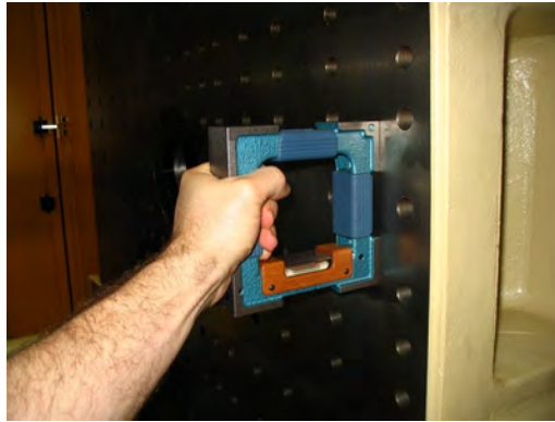
Figure 5-35: Box Level Measurement on Stationary Platen (L5)
