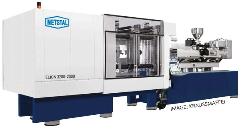
**Above: The dry-cycle times of the Netstal Elion have been reduced by up to 0.2s across the entire model range**
