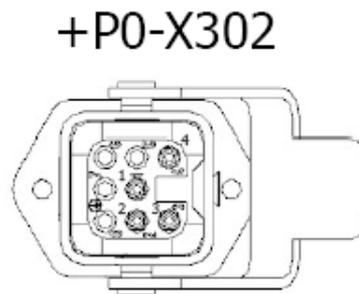
**Figure 2-14 Screw Position Cable Potentiometer Analog Input - X302 Connector**
