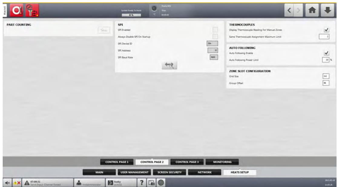
Figure 5-5 Heats Setup - Control Page 2 Tab (Integrated System)
