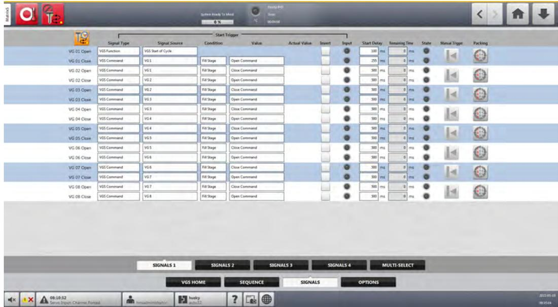
Figure 6-4 Valve Gate Sequencer Signals Screen
