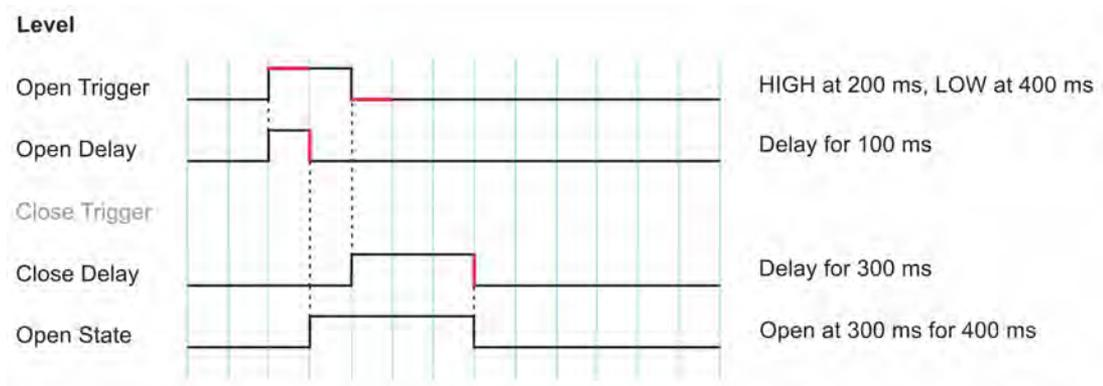
Figure 6-16 Level Cycle Example
