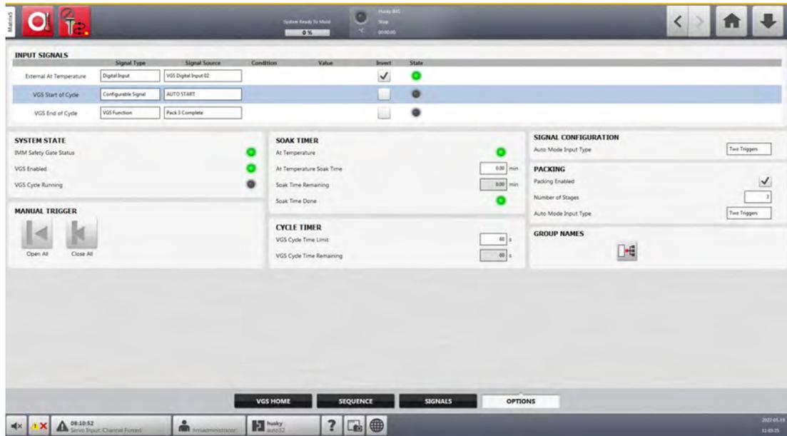
Figure 6-14 Valve Gate Sequencer Options Screen
