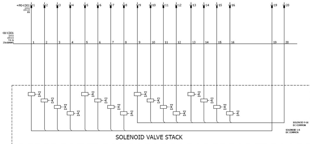
Figure 2-13 X301 Flying Lead Electrical Schematic, 16 Solenoid Outputs
