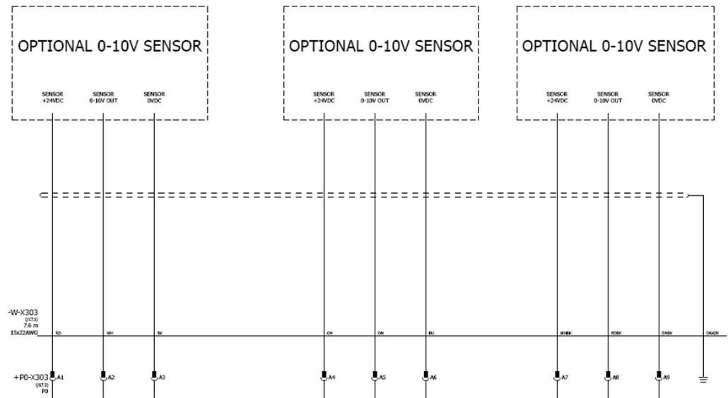
Figure 2-18 W-X303 Cable Electrical Schematic, 0-10 V Signals
