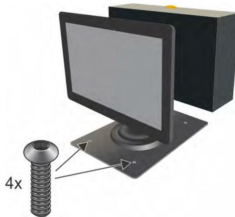
**Figure 2-6** Display Module - Attachment
