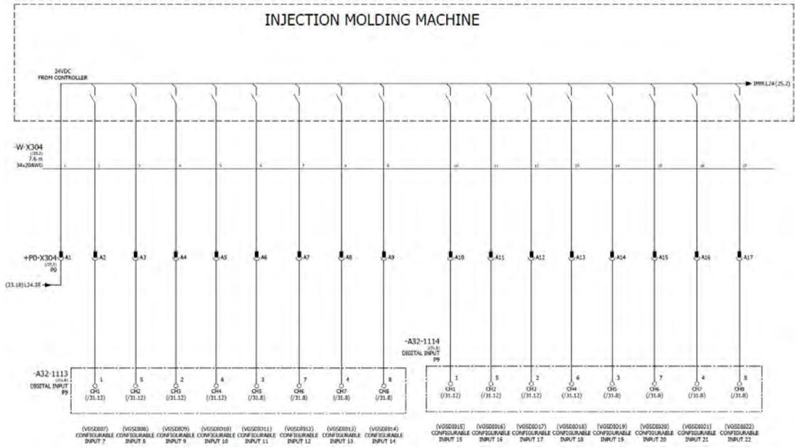
**Figure 2-21 W-X304 Cable Electrical Schematic (1)**
