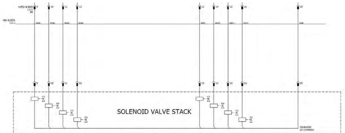
Figure 2-25 X305 Flying Lead Electrical Schematic, Solenoid Outputs 25-32
