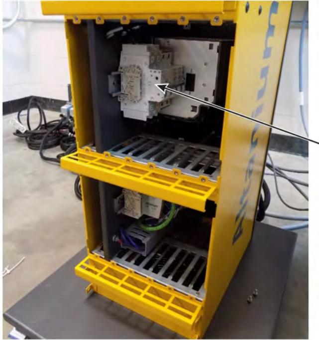
**Figure B-2**      **Circuit Breakers Location - Second Bay**
