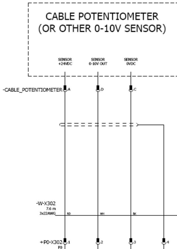
Figure 2-16 W-X302 Cable Potentiometer Cable Electrical Schematic
