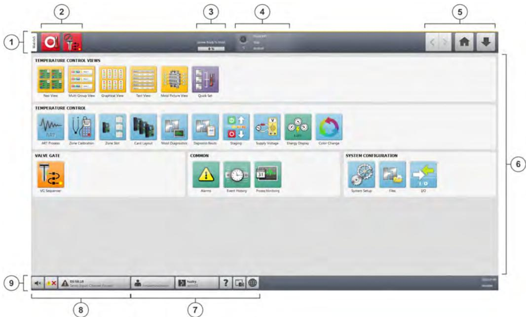
**Figure 3-1 Altanium Controller Home Screen with Valve Gate Sequencer - Integrated Temperature System**
