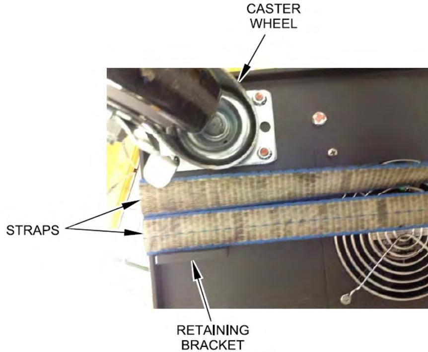
**Figure 2-3 Straps - Correct Position**
