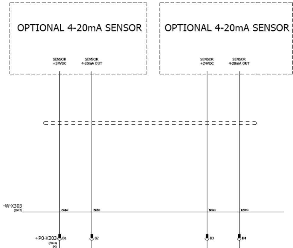
Figure 2-19 W-X303 Cable Electrical Schematic, 4-20 mA Signals
