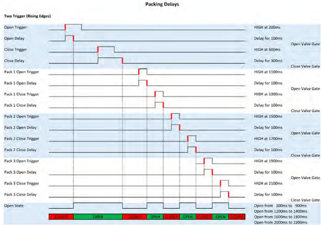
**Figure 6-9 Packing Delays Example**
