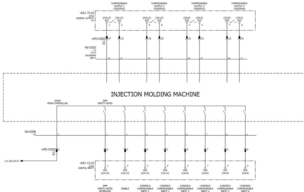
**Figure 2-10 W-X300 Cable Electrical Schematic**
