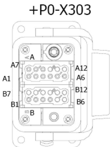
**Figure 2-17 Additional Analog Inputs - X303 Connector**
