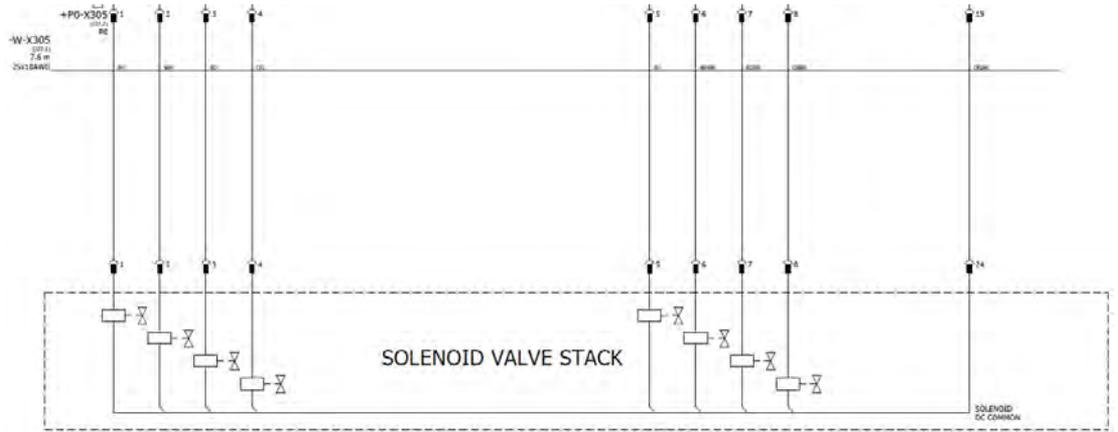
Figure 2-24 X305 Flying Lead Electrical Schematic, Solenoid Outputs 17-24
