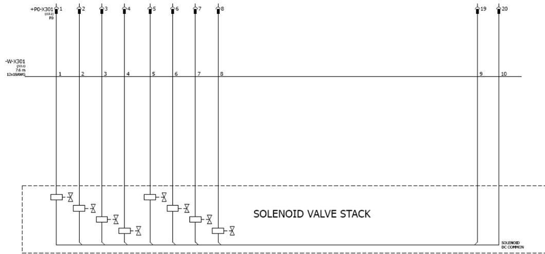
Figure 2-12 X301 Flying Lead Electrical Schematic, 8 Solenoid Outputs
