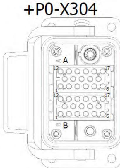
**Figure 2-20 Injection Molding Machine Interface - X304 Connector**
