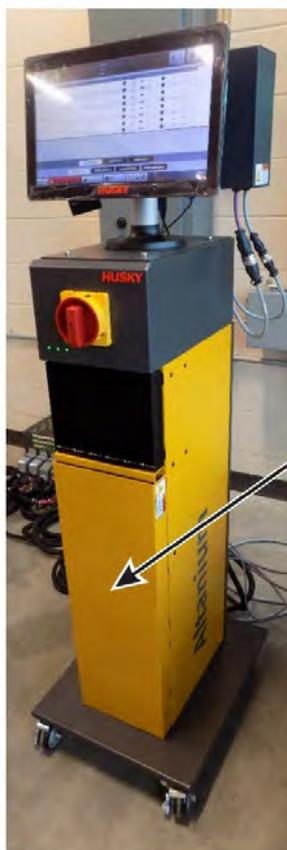
**Figure B-1 Air Duct Cover**
