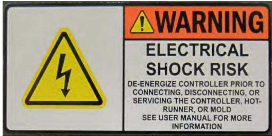
Figure 1-1 Hazard Voltage Warning Example
