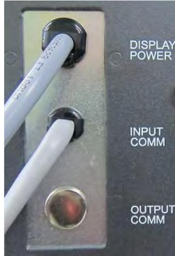
Figure 2-26 Display Power and Temperature Control Connections
