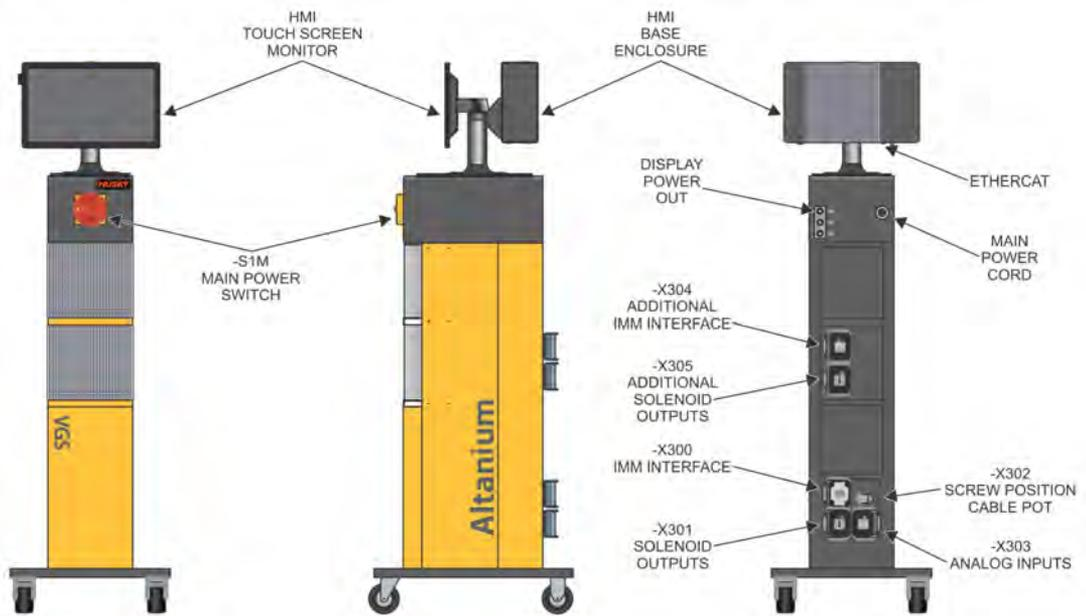
**Figure 2-1 VGSC Controls, Connectors, and Parts Identification (Standalone System)**
