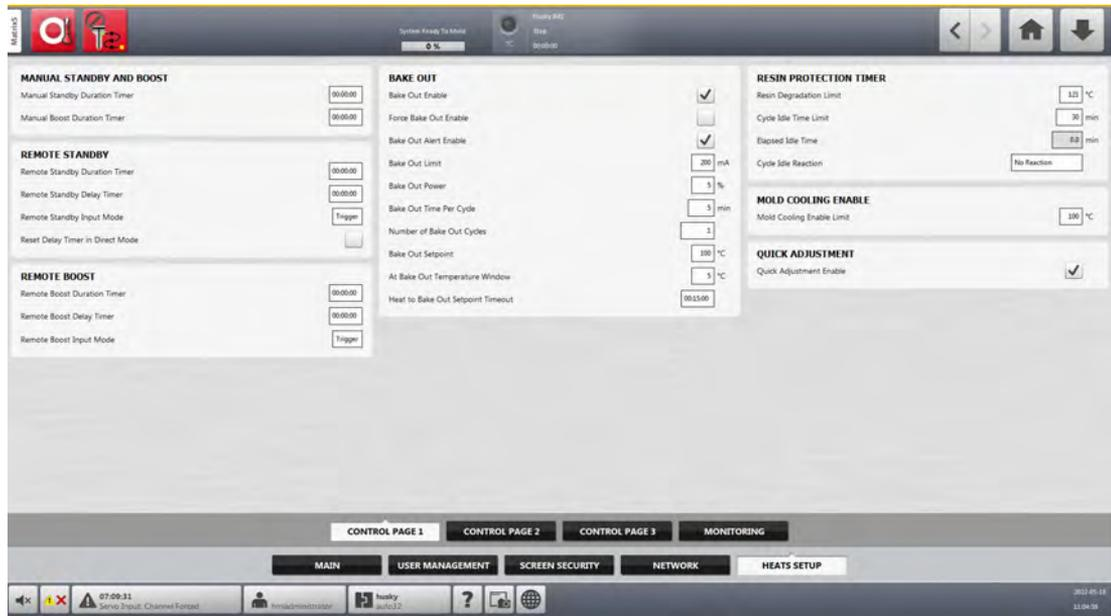
Figure 5-4 Heats Setup - Control Page 1 Tab (Integrated System)
