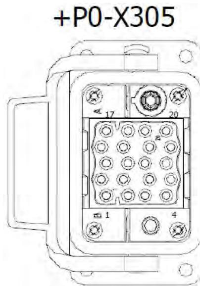
**Figure 2-23 Solenoid Outputs - X305 Connector**
