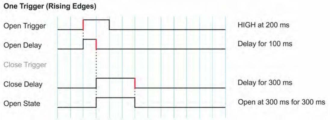
Figure 6-17 One Trigger Cycle Example
