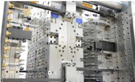
Fig. 1: 96+96-fold stack mold for 5ml centric luer slip barrel
