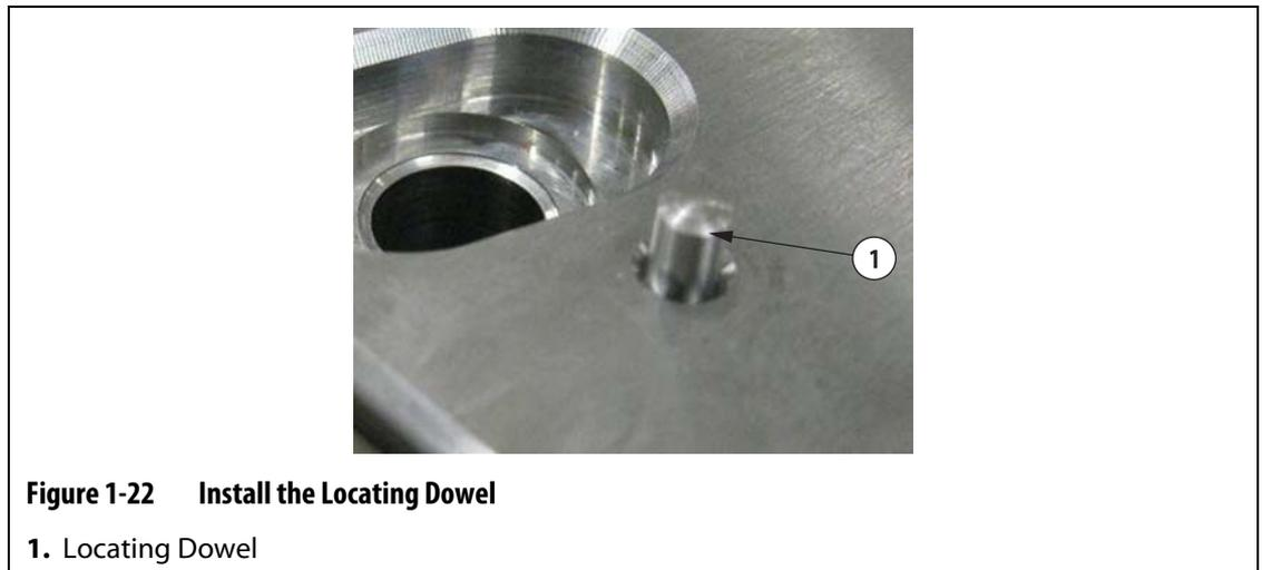
2. Place the locating dowel into the locating hole on the manifold.
