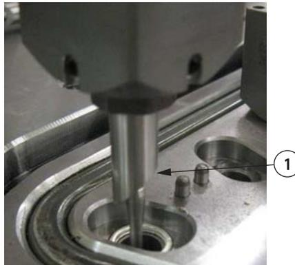
**Figure 1-24 Install the Actuator Assembly**
