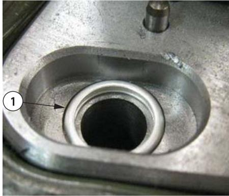
**Figure 1-23 Install the Crush Ring**
