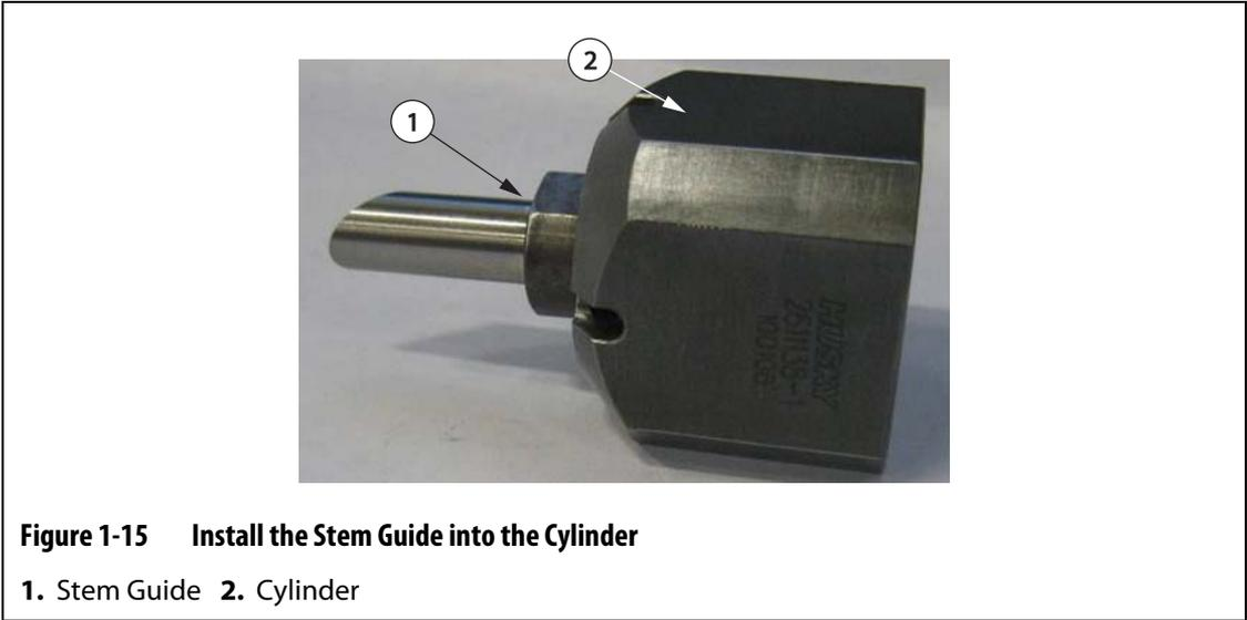
**11.** Using the snap ring tool, place the snap ring over the top of the stem guide that is now inside of the cylinder.
