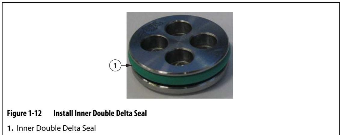
3. With the piston counter-bore side up, place the green inner double delta seal into the groove around the metal piston's rim. No tools are required.
